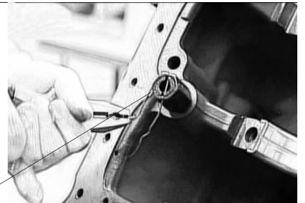
Fig 5-2 Pressure Limiting Valve of Oil Pump
